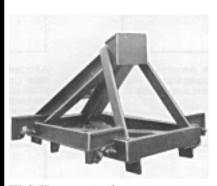
W-C-H recognized many years ago that a cushioning effect was achieved if a railroad car-stopping device was allowed to dissipate car momentum by shoving ties and ballast. Transferring impact into the ties and ballast reduces damage to lading, car, rail and bumper. Our Type WP Bumping Post, pictured here, employs this principle and has been in use since the late 1950's.
