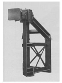
The building was not long enough to accommodate railroad cars and a Bumping Post, too. To solve this problem, we designed a unit with a below-ground super-structure and an extended face. Installed outside, stability is provided by the below-ground portion of the Bumping Post and the extended face reaches through the wall to contact railroad car couplers.
