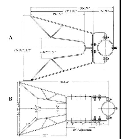
Properly installed, the W-C-H High Wind Gate Arm Support can significantly reduce wind caused knock-downs of breakaway gate arms. Unique features such as
