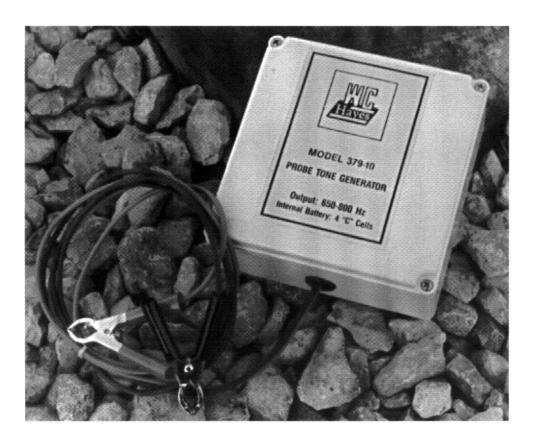
The Western-Cullen-Hayes Model 379 Probe Tone Generator is a battery powered (6VDC, 80 mA continuous duty, four "C" cells) unit used to generate an AC tone (650-800 Hz) into non-coded DC track circuits, for the purpose of using the Model 370 Track Circuit Probe to locate trouble spots.
